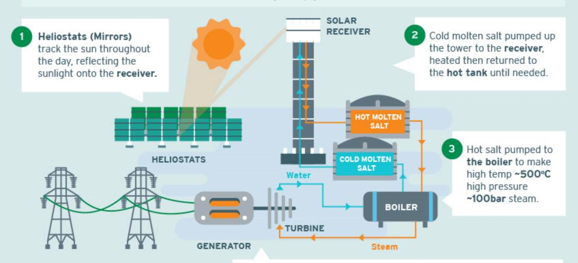
4 Steam turns the turbine to drive the generator to make electricity.
