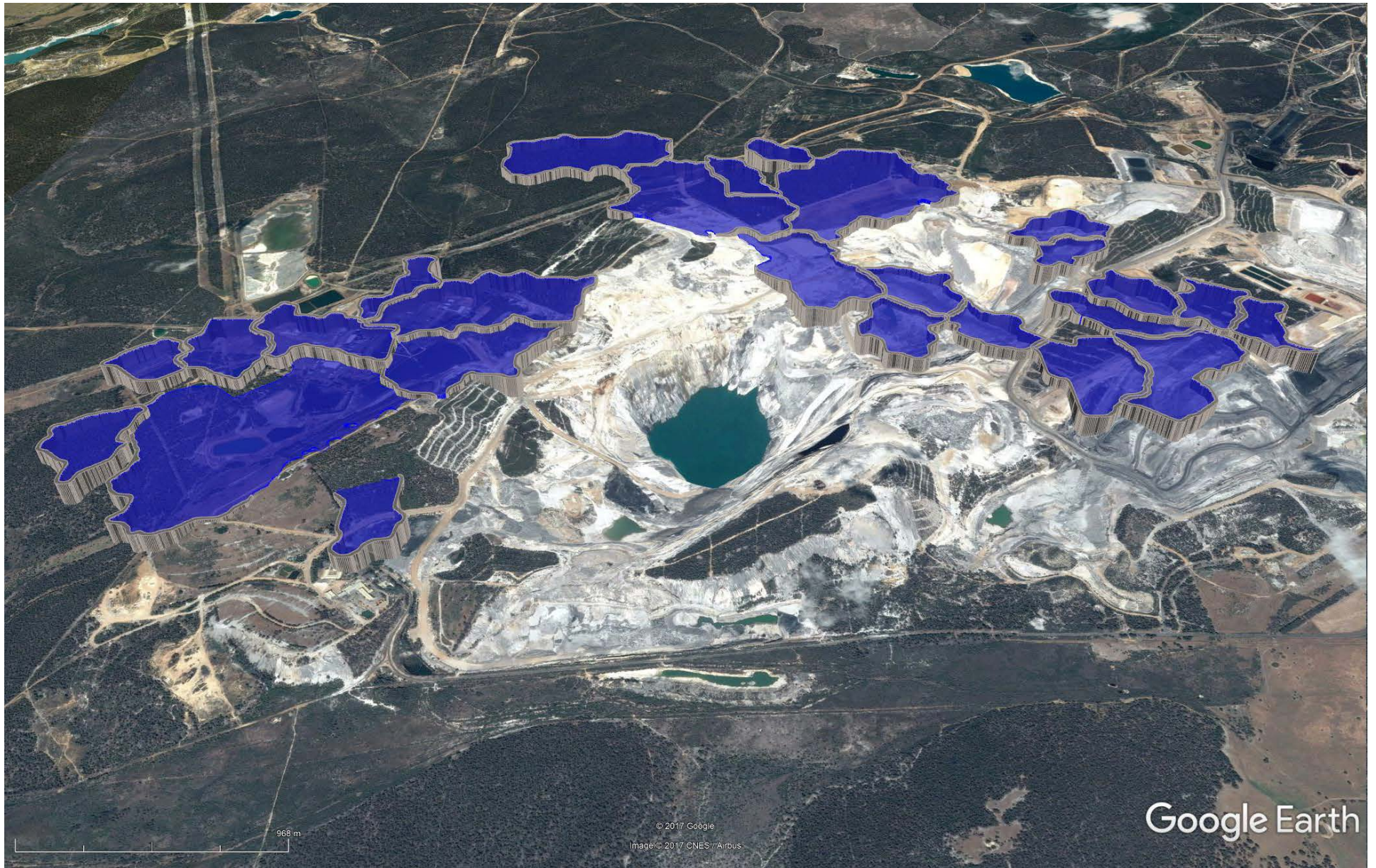
Figure 15: Potential PHES upper reservoir sites at Collie, WA, with 200 m head into the pit and a good volume of stored water.
