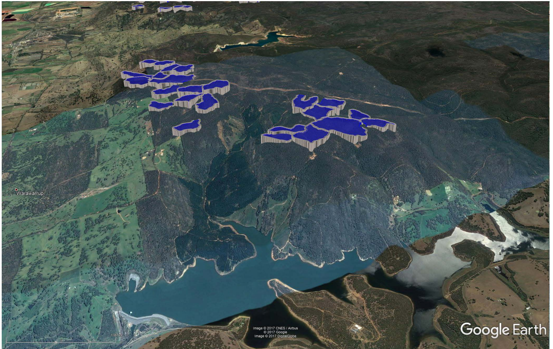
Figure 16: Potential PHES upper reservoir sites near Harvey, WA. The existing reservoir at the bottom of the image could be incorporated into a PHES system.
