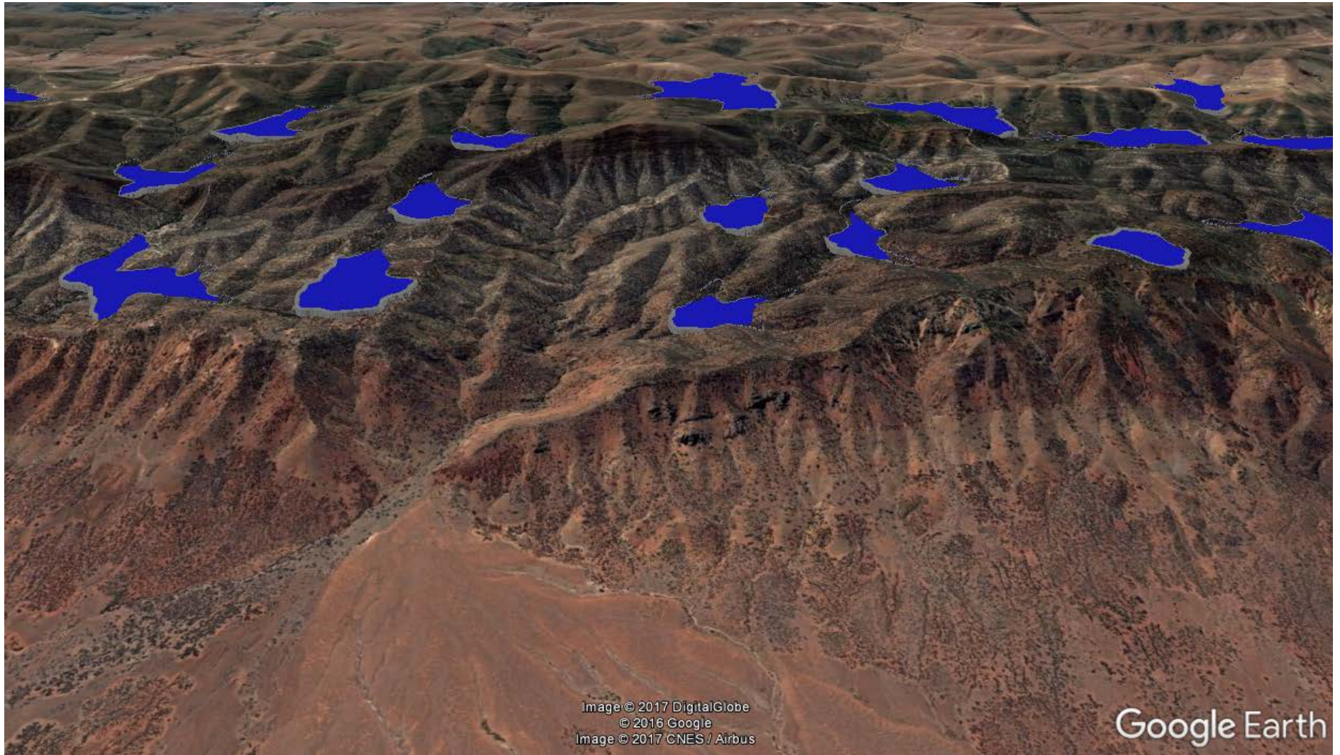
Figure 9: Potential PHES upper reservoir sites in Region A, east of Port Augusta. The lower reservoirs would be at the western foot of the hills (bottom of the image).
