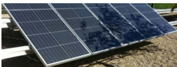
Figure 2: SLIVER modules undergoing outdoor testing to measure the effect of shading on power output. SLIVER modules display substantially better shade tolerance than most other commercial modules. Source: Transform Solar
