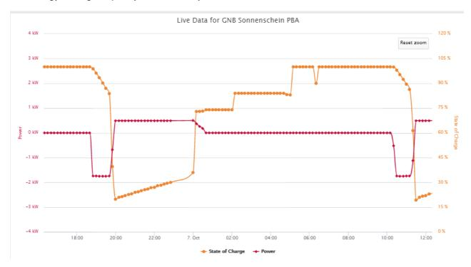
Figure 15 GNB Lead Acid battery SOC Recalculation under load
