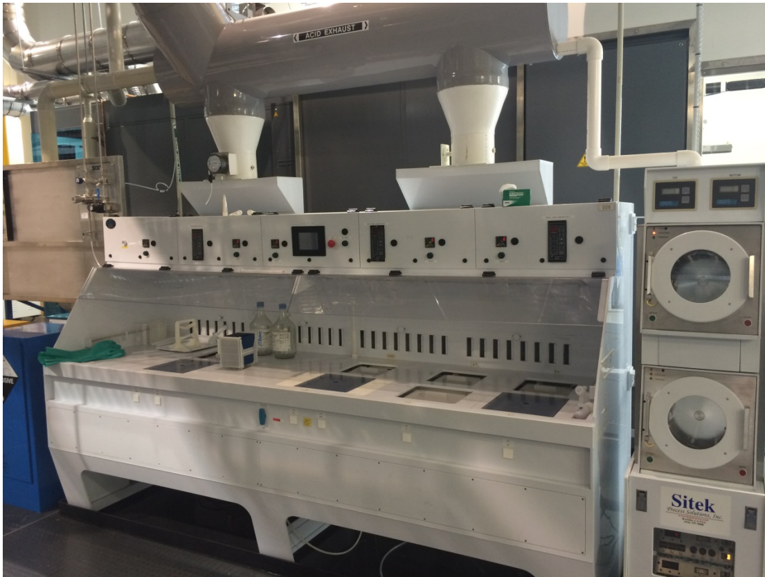
Figure 6: Chemical baths for general chemical processing and cleaning with spin-dryers shown on the right.
