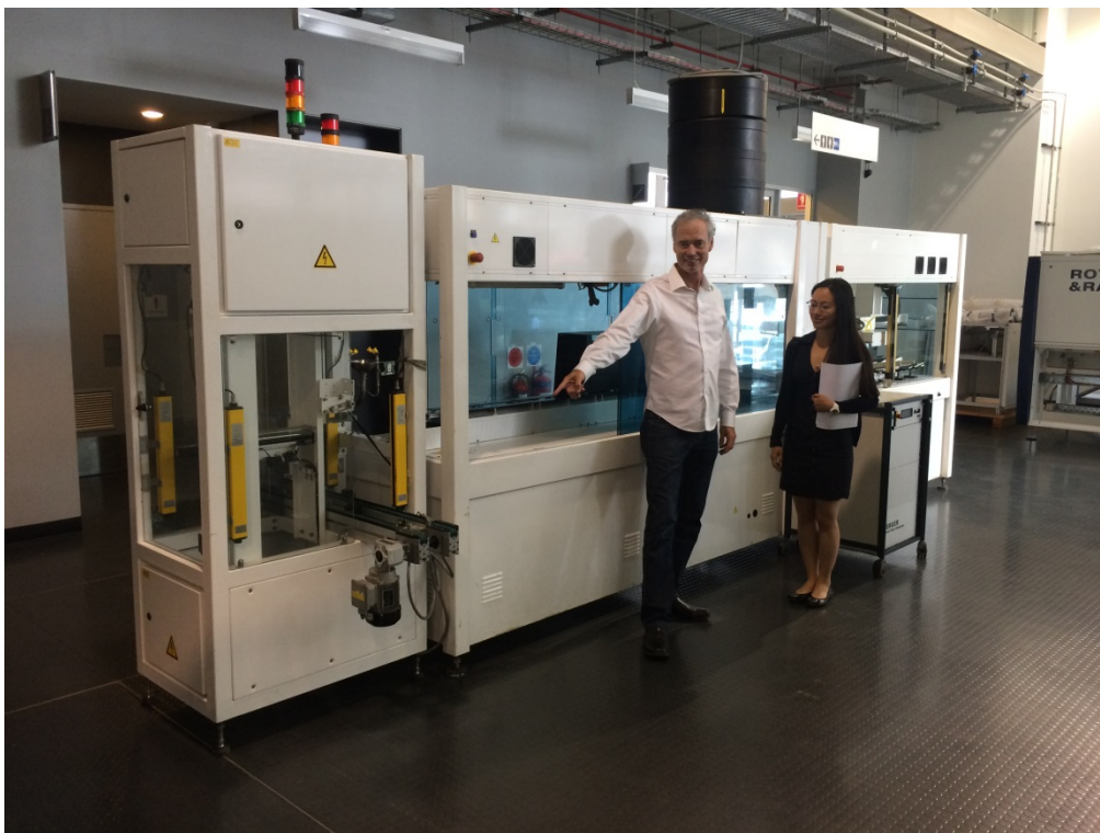
Figure 8: Following completion of device fabrication, cells are tested in the automated testing station manufactured by Bacini
