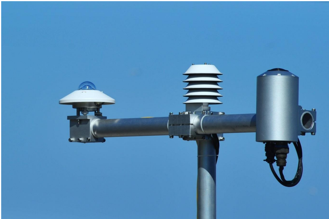
Figure 1: The commercially available CloudCAM (right) with attached pyranometer (left) and met station (centre)
