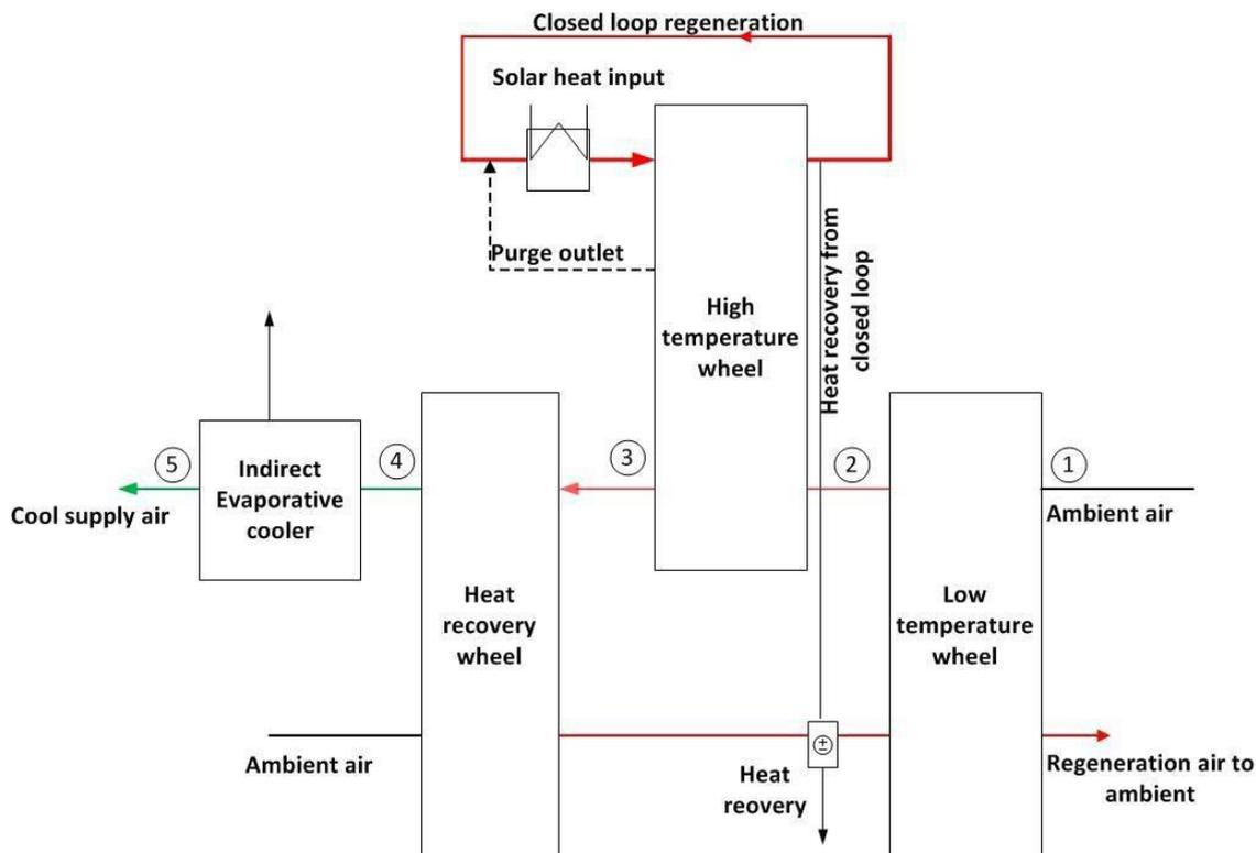
**Figure 1** *Process diagram for two stage desiccant air conditioning system. The system incorporates a heat cascading design for increasing the efficiency of the air conditioning system.*
