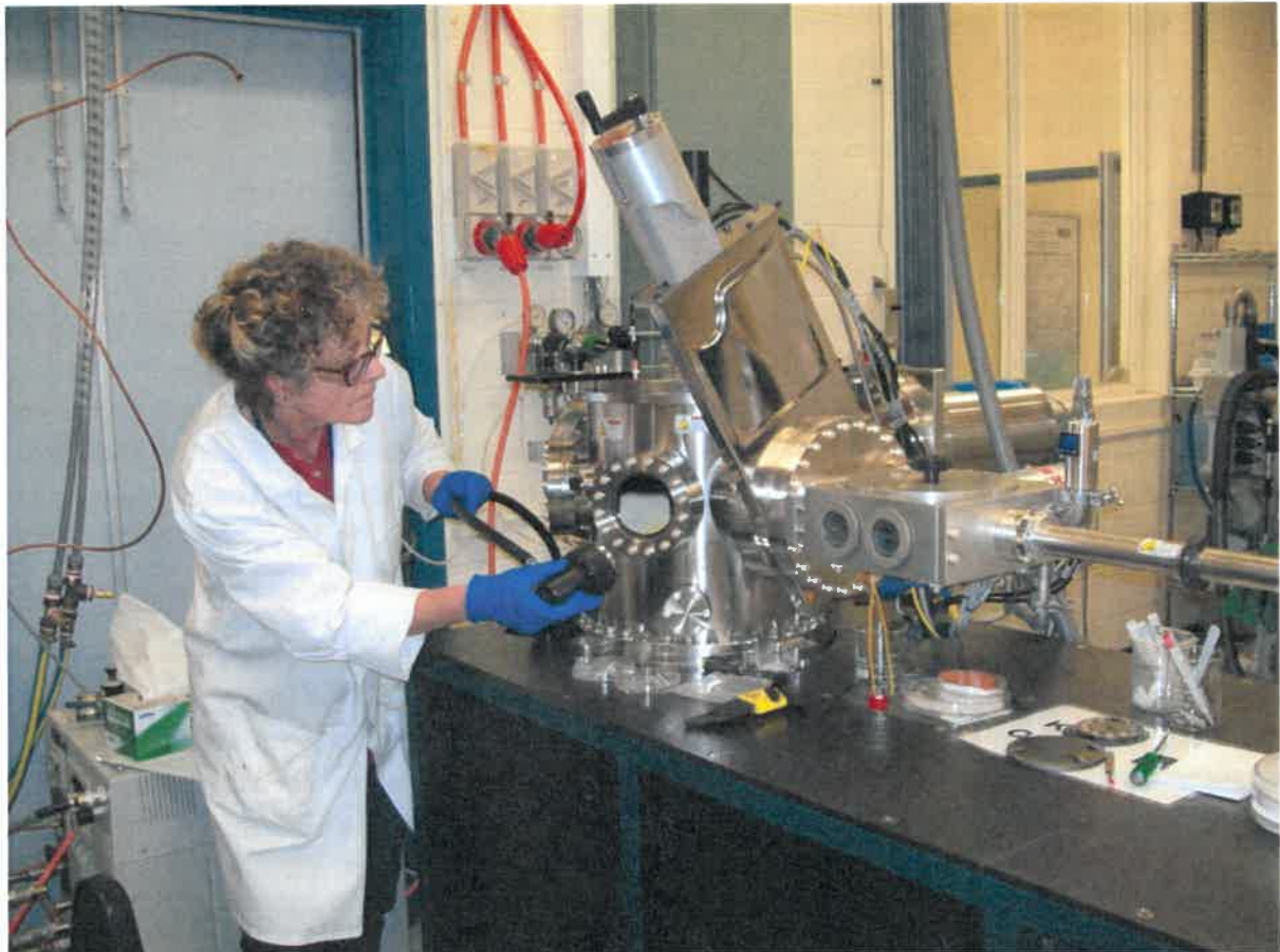
Sputtering was one of the promising approaches used for depositing novel dielectric films for coating the solar cells.
