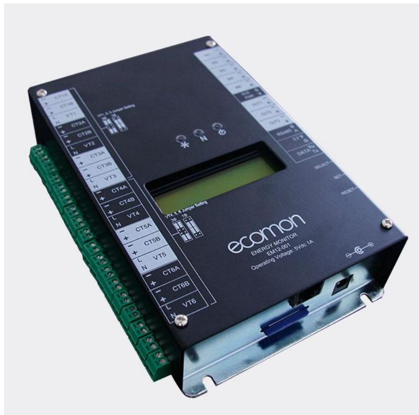
Figure 1. An example of the ecomon energy monitor installed in volunteer households.
