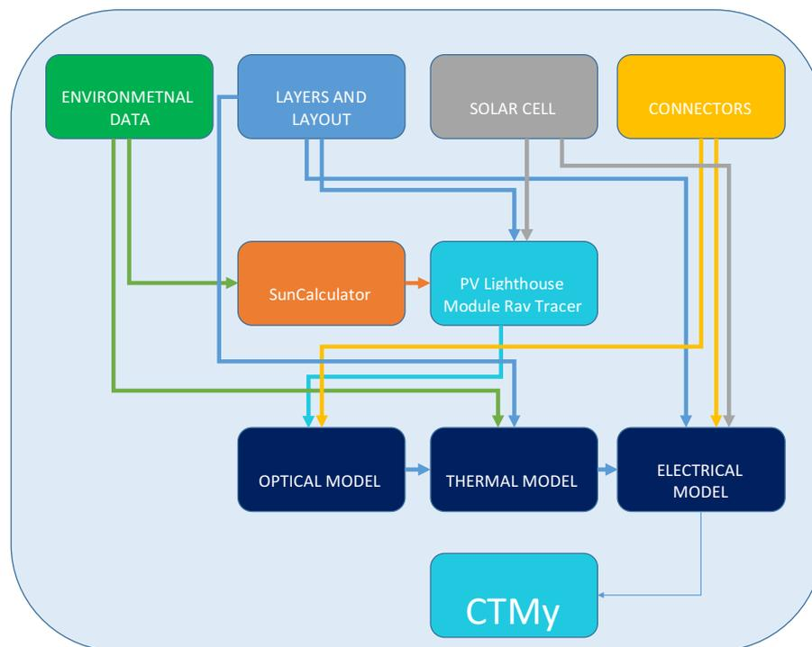
**Fig. 1** Schematic of the CTMy model depicting the data flow and calculations performed to determine location specific losses.
