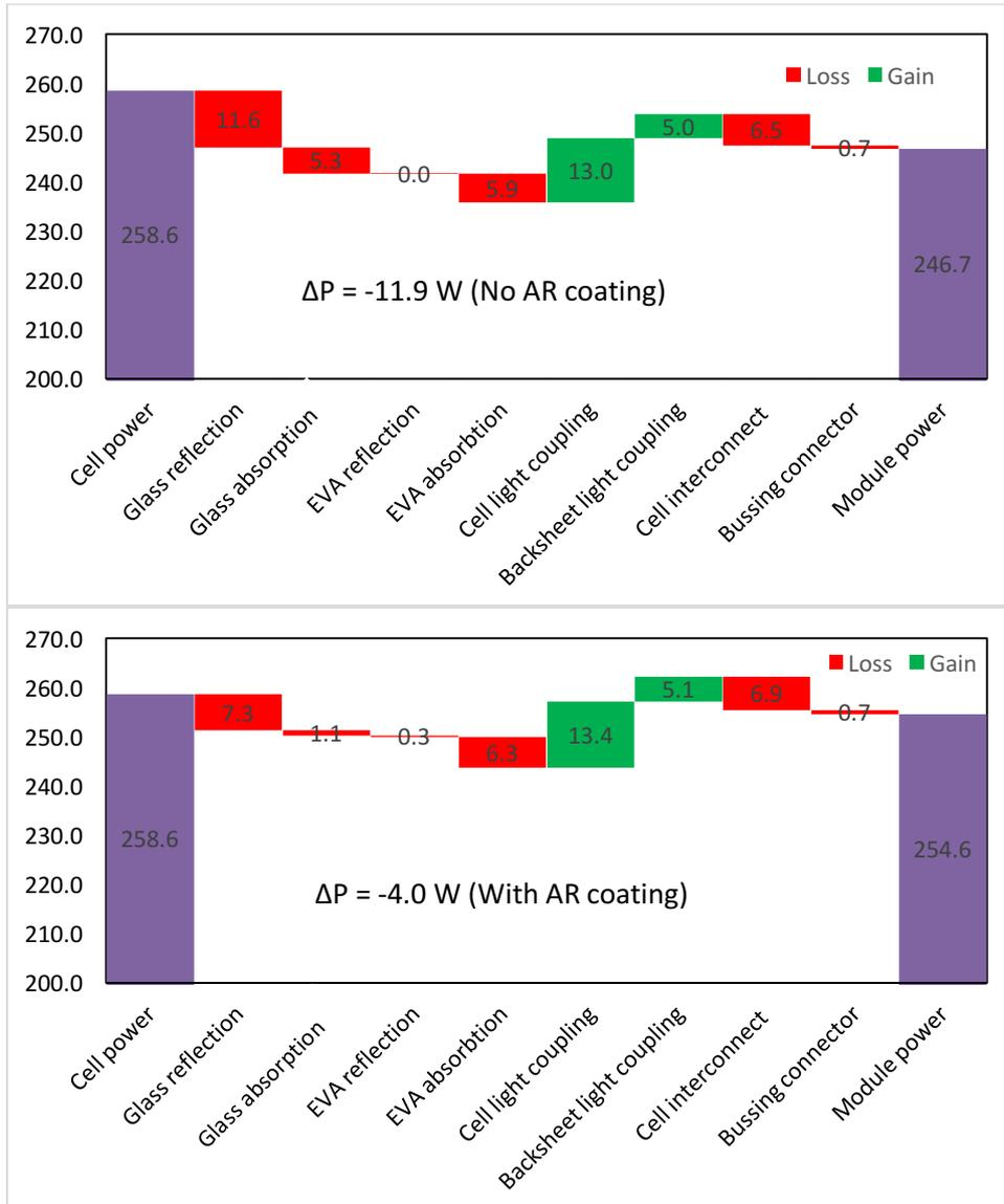
Figure 2: Waterfall diagram for power gains and losses for a Tindo Solar module with (top) and without (bottom) anti-reflection coating on the glass. Analysis based on a procedure developed by Haedrich et al (Search: Unified methodology for determining CTM ratios: Systematic prediction of module power)
