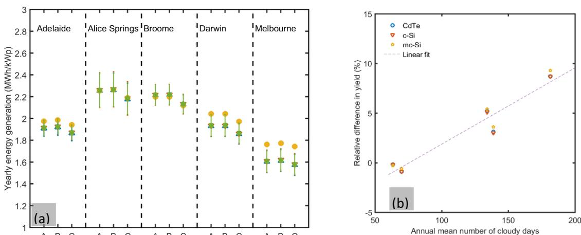
Fig. 2. (a) Yearly energy generation and 95% confidence intervals calculated for four combinations of irradiance and temperature datasets and for the three module technologies (A, B, C). (b) Relative difference of ASEIS yield (●) to BoM one-minute yield (▲) as a function of the annual mean number of cloudy days.
