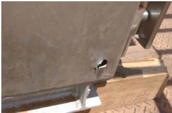
Left and right: Examples of transit damage to switchboards for the SETuP program
