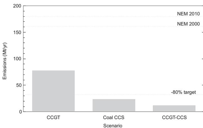
**Fig. 2.** Annual emissions from different fossil fuel scenarios for electricity generation. Horizontal lines show emissions produced from NEM operations in the year 2000 and 2010. The level required to reduce emissions by 80% is also shown.
