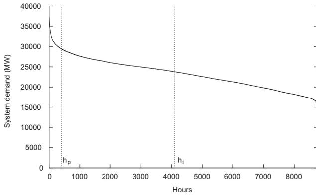
**Fig. 1.** System-wide load duration curve for the NEM in 2010 with  $h_p$  and  $h_i$  chosen arbitrarily for illustration.  $h_p$  and  $h_i$  are the number of hours of peaking and intermediate plant operation, respectively. Data source: AEMO.
