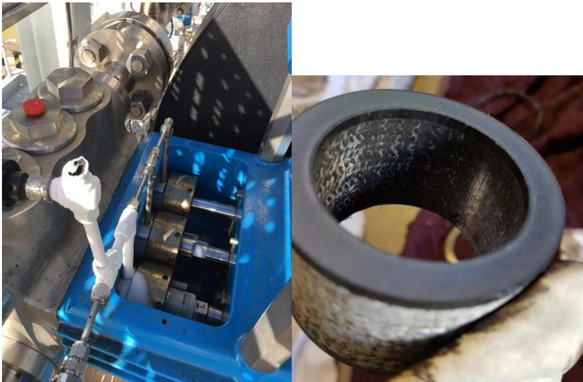
**Figure 3 LHS - sCO<sub>2</sub> pump in operation showing expanding CO<sub>2</sub> freezing the vent pipe. RHS - Compression packing from the pump plunger.**
