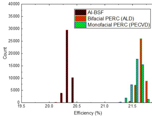
Figure 1: High-volume production data for the incumbent Al-BSF technology and PERC solar cells with a monofacial and bifacial aluminium oxide layer. It can clearly be seen that the solar cells with the bifacial aluminium oxide layer show a better performance compared to the monofacial aluminium oxide layer while the production costs of the bifacial aluminium oxide are lower.
