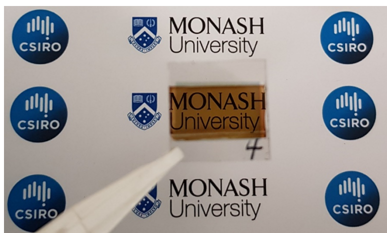
Figure 1. Semi-transparent perovskite solar cell with a Monash University and CSIRO backdrop. (Source: Jae Choul Yu)
