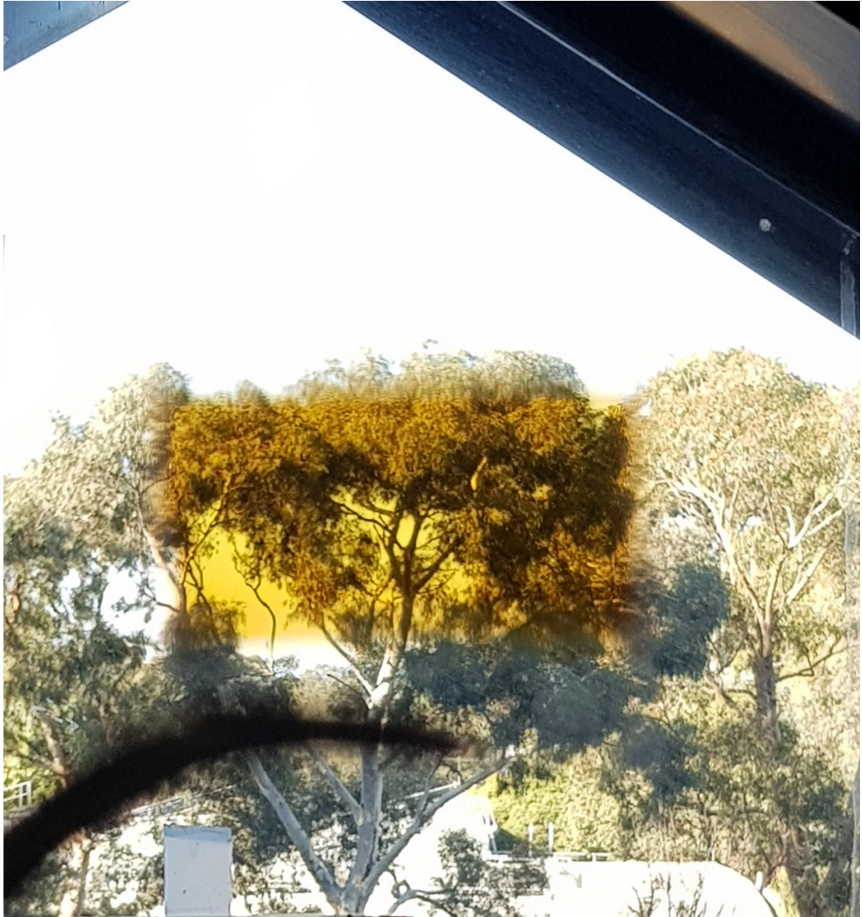
Figure 2. Semi-transparent perovskite solar cell with natural landscape background. (Source: Jae Choul Yu)
