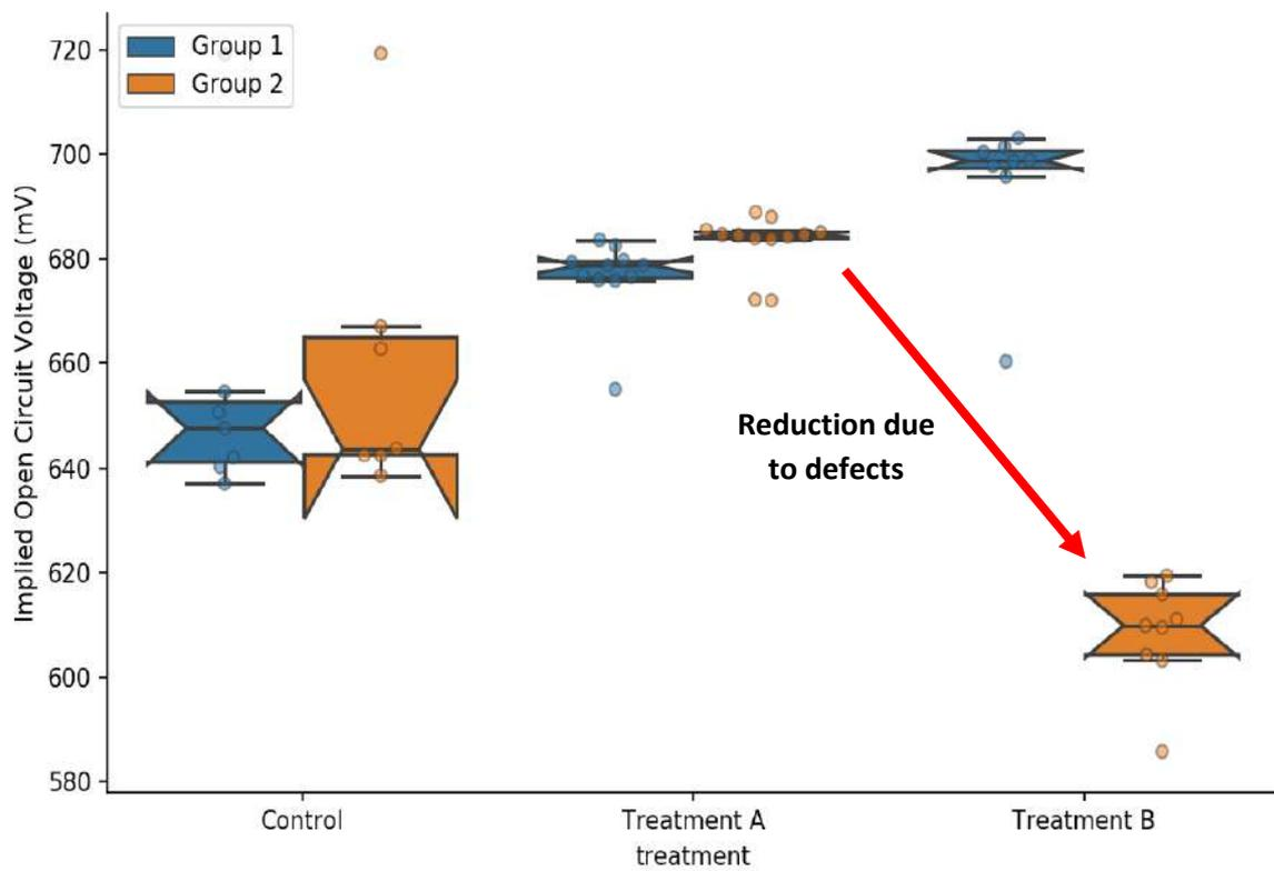
Figure: A severe reduction in the implied open circuit voltage, a property used to measure n-type silicon wafer quality, is observed due to the presence of oxygen-related defects.
