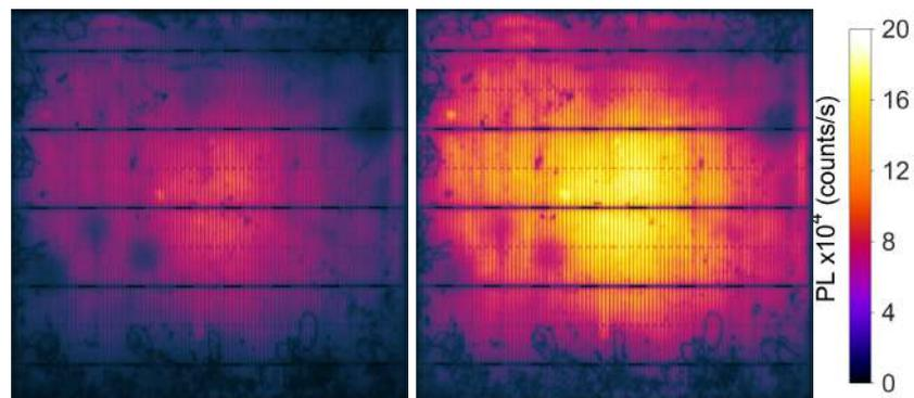
Figure: Photoluminescence images of a n-type silicon solar cell before (left) and after (right) a treatment to control hydrogen in the silicon. The bright regions indicate higher material qualities.
