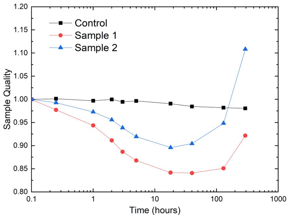
Figure: Change in material quality for all three different n-type silicon samples that were tested under 1 sun equivalent light intensity at 75 °C. The control sample (without diffusion) was not degraded; sample 1 and 2 with boron and phosphorous diffusion respectively were degraded under 1 sun and 75 °C.
