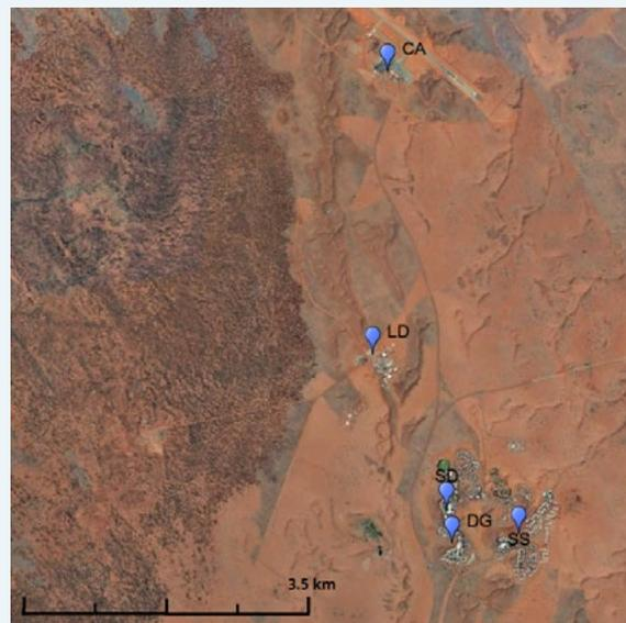
**Figure 2: Geographical distribution of the PV arrays in the 1.8 MW<sub>p</sub> Yulara system, where CA = Connellan Airport (106 kW<sub>p</sub>), LD = Laundry (328 kW<sub>p</sub>), SD = Sails in the Desert (107 kW<sub>p</sub>), DG = Desert Gardens (1060 kW<sub>p</sub>) and SS = Service Station (227 kW<sub>p</sub>)**
