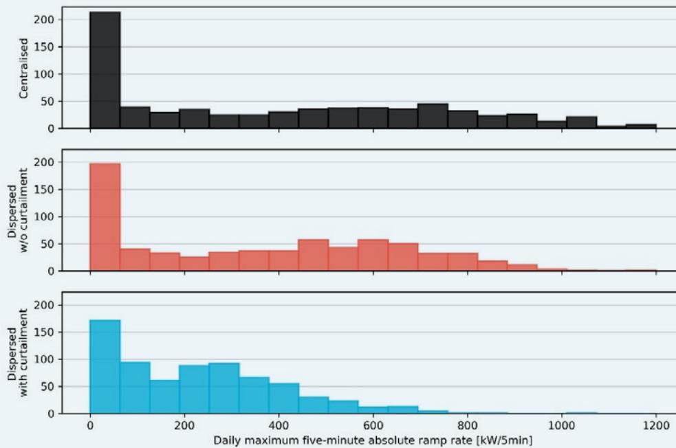
Figure 7: Histogram of the daily maximum 5-minute ramp rates at Yulara's PV power station based on measured and calculated data, observing the impact of dispersion and curtailment.
