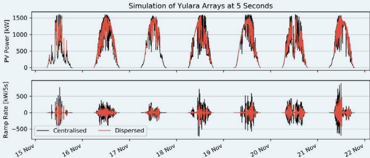
Figure 4: Comparison of the variability in modelled power output of a geographically dispersed system (red) to a centralised system (black) based on the 1.8 MWP Yulara PV plant, simulating data at a 5-second timescale
