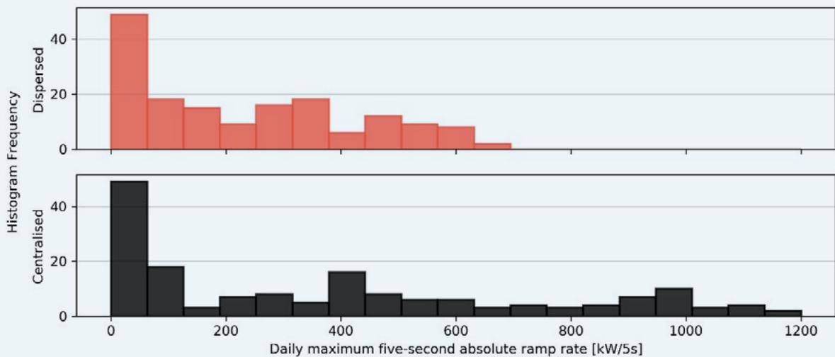
Figure 5: Simulated power variations encountered by dispersed (red) and centralised (black) array layouts. Each histogram bin shows the number of days over a 10-month period in which a particular maximum absolute ramp rate was observed.
