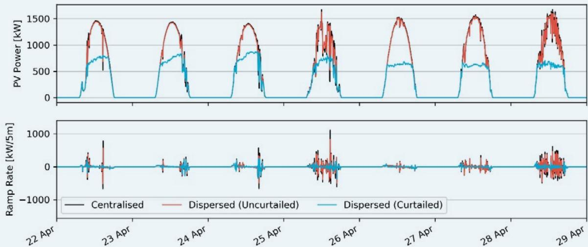
Figure 6: Comparison of the operation of the Yulara array (blue is actual operation: Dispersed with curtailment), compared to uncurtailed dispersed (red) and uncurtailed centralised (black) operation.
