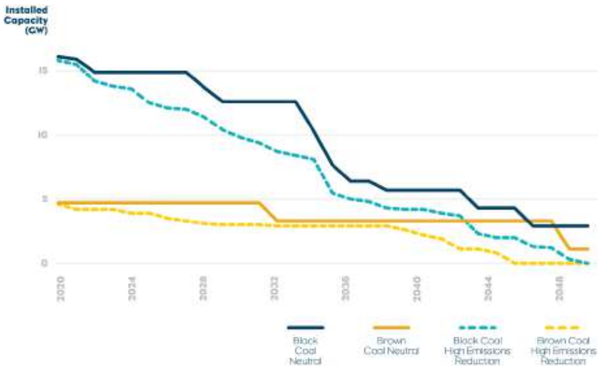
Figure 19 Retirement of coal-fired generators in neutral scenario and high emissions reduction sensitivity 110
