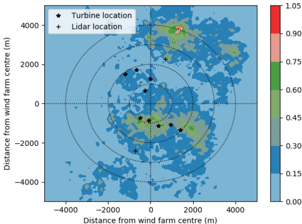
*Figure 2* LIDAR (crosses) and turbine (stars) placement relative to the geographic centre of the Kiata Wind Farm. Shading shows relative probability of air parcels in the flow being in a location five minutes after measurement.
