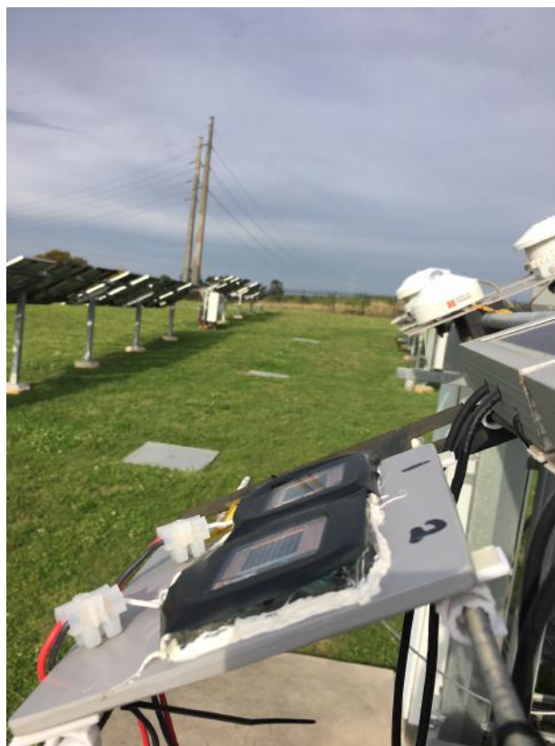
Figure 1: Tandem cell being tested outdoor
