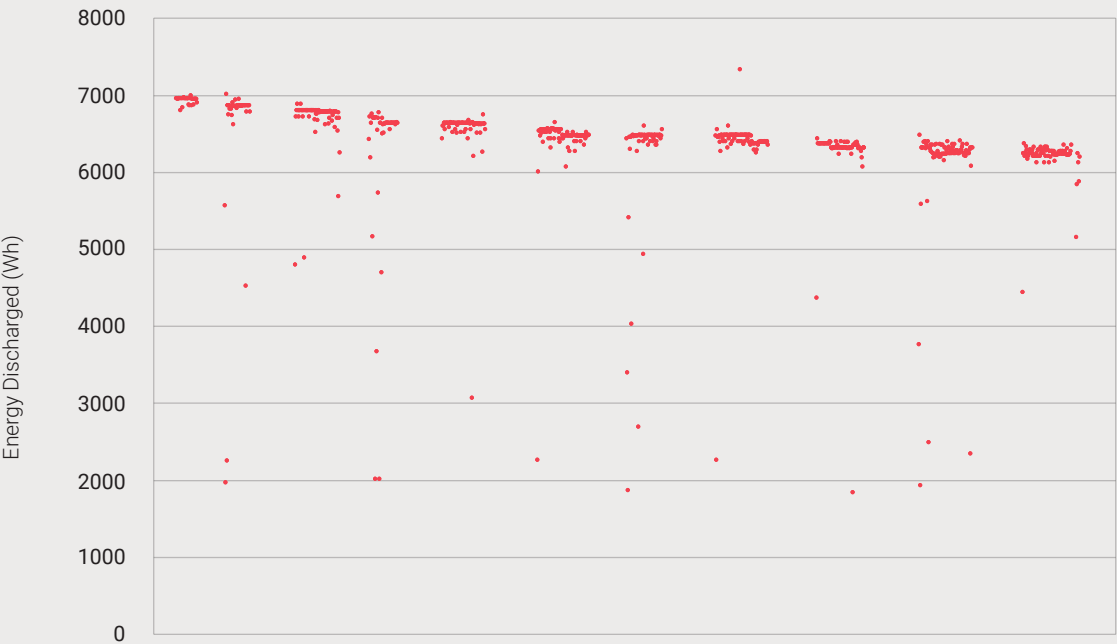
Figure 7. Energy discharged per cycle by the LG Chem RESU HV battery pack
