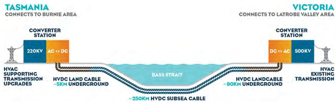
Figure 9 Schematic representation of Marinus Link
