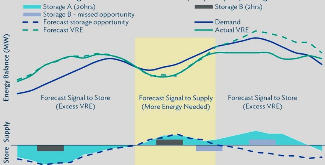
**Figure 4.** Illustrative storage operation<sup>8</sup> with an imperfect forecast for wind and solar (VRE)
