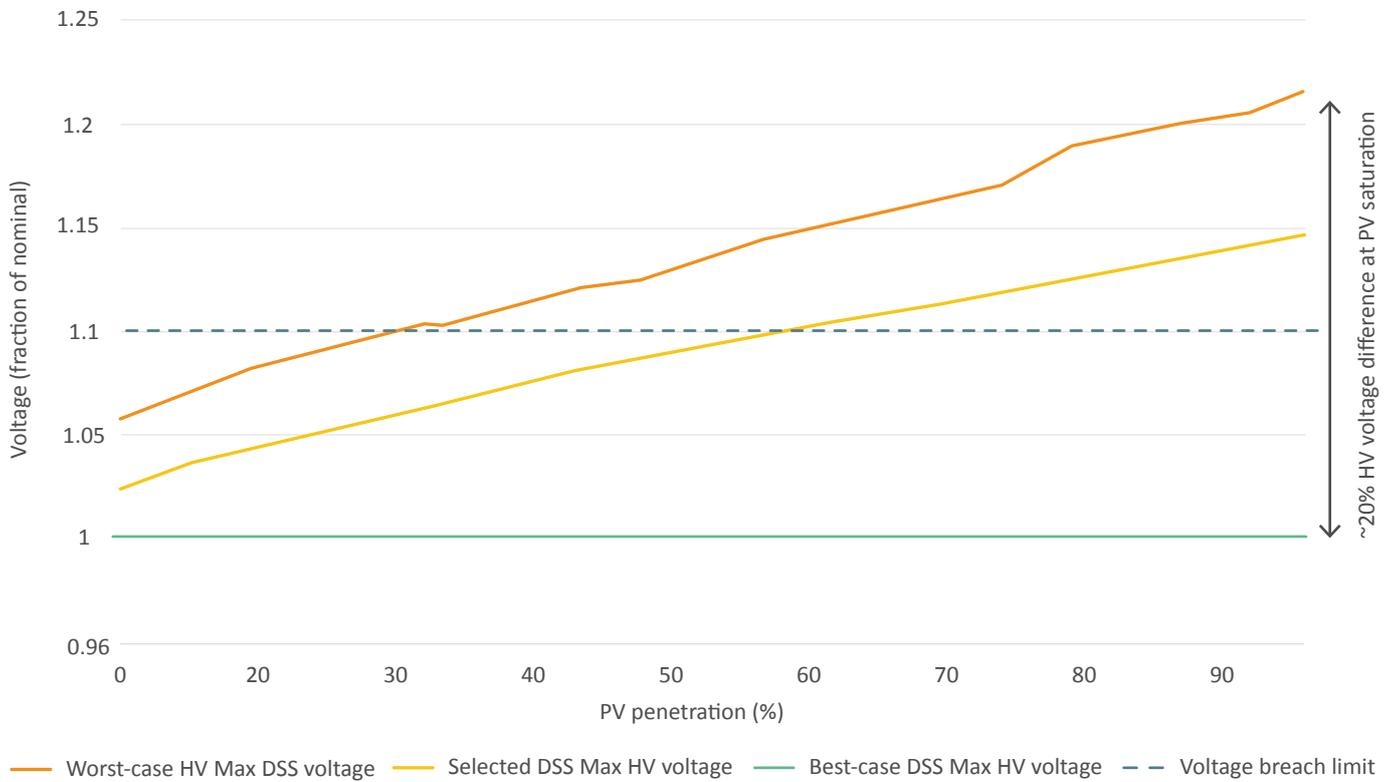
**Figure 12 • Maximum theoretical HV voltage rise for three DSS locations on an Urban HV feeder**
