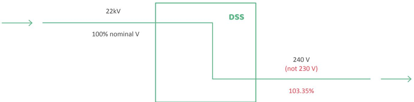
The result of this effect is equivalent to a loss of more than one 'buck' tap on the transformer in question, which can represent a considerable portion of the available +10% headroom. Of the 10 example LV networks, eight were equipped with transformers exhibiting this issue.
