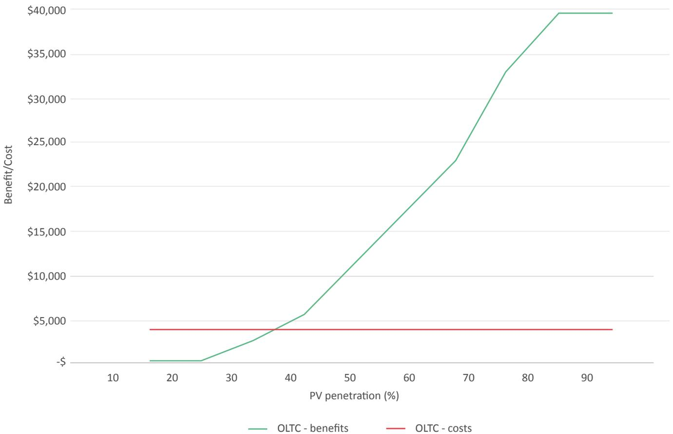
Figure 18 shows that the cost of OLTC is independent of the PV penetration so remains flat to saturation. This is different to customer-side measures such as behind-the-meter batteries and smart inverters, where the cost increases with PV penetration. As PV penetration increases, the benefit of additional PV generation eventually outweighs the costs at around 36% PV penetration, resulting in positive net-benefits.
