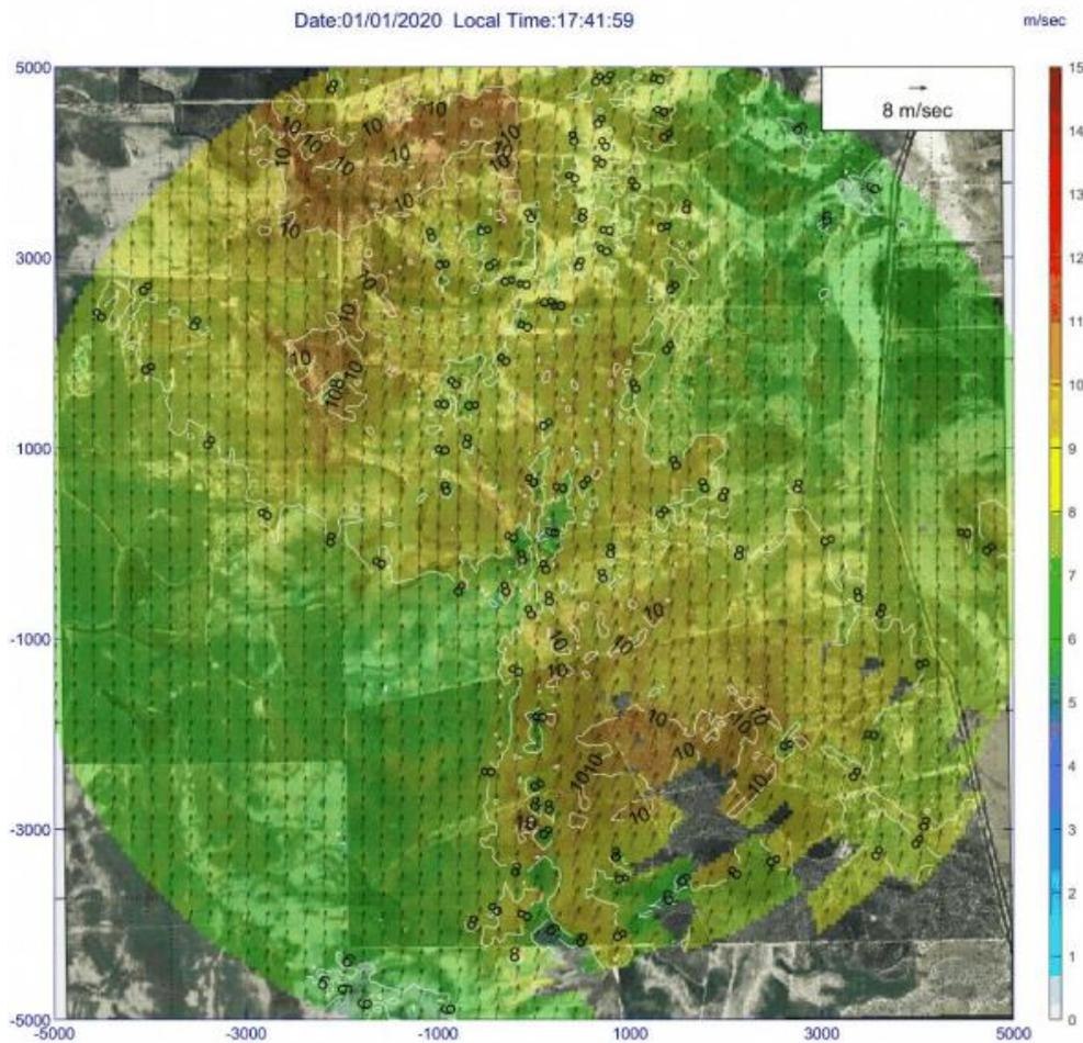
*Figure 2. Example of 10-minute average wind speed terrain following windfield at 40 M agl. The structure and complexity of the windfield over the 78.5 km<sup>2</sup> area is clearly illustrated in the plot. An understanding of atmospheric dynamics and the effect of topography on flow behaviour upstream of the windfarm is crucial for securing accurate power forecasts.*
