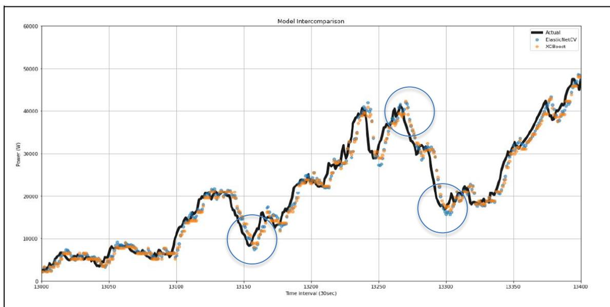
Figure 1. Example of Neural network forecaster skill demonstrating the lag between two forecasters (blue and orange trace), and actual power production (black trace) during a ramp up event. Whilst the forecasts are in reasonable agreement with actual power output for significant periods of time, they fail to capture important turning points in the overall trend with the required resolution to be of use in operational forecasting (circles).
