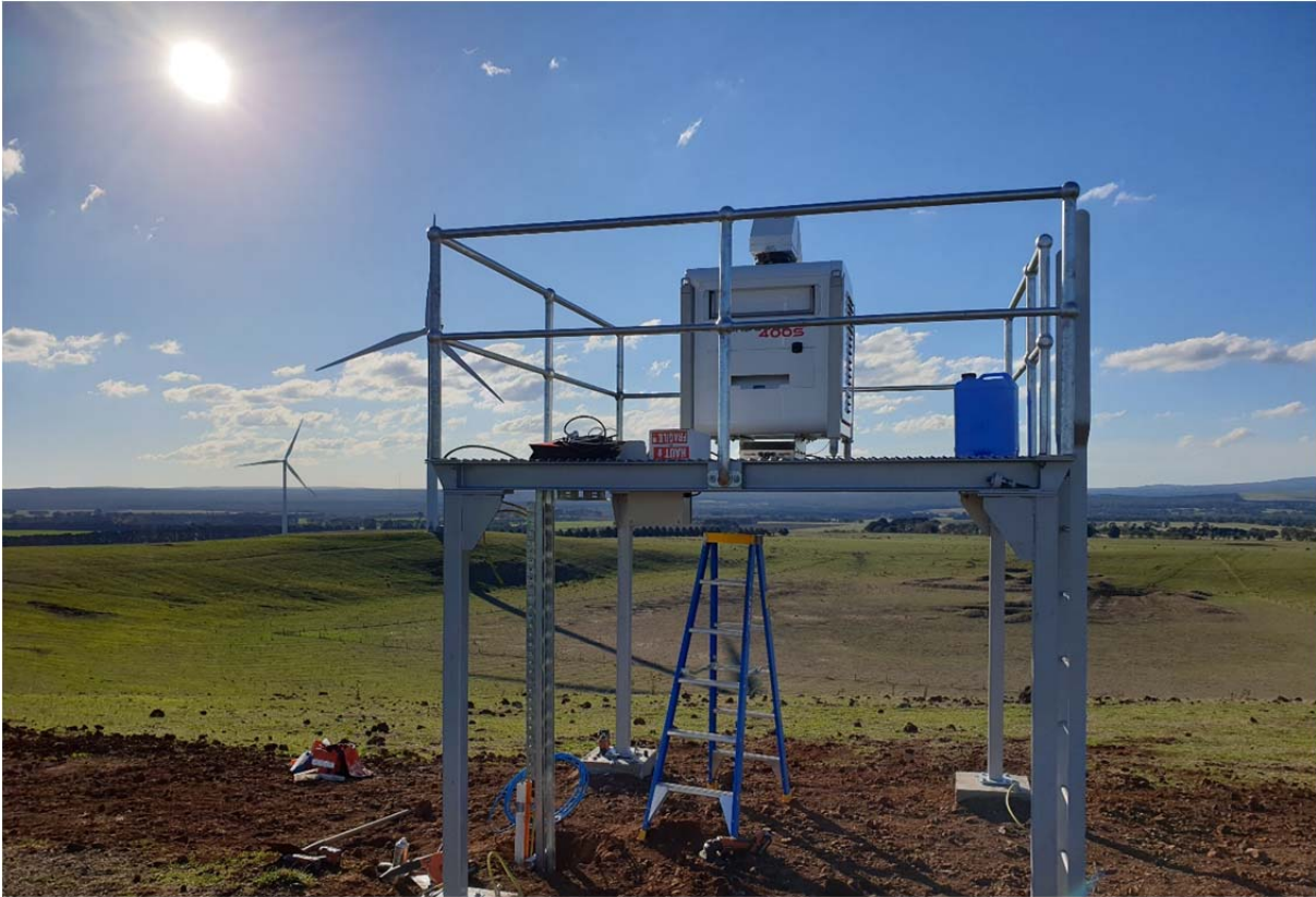
Figure 1: Picture of the Leosphere Windcube 400S Scanning LIDAR system atop Mt Mercer
