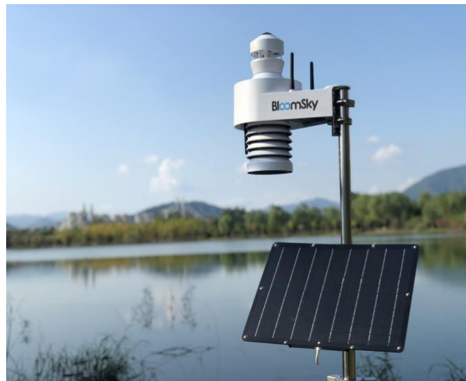
Example sky-imager installation solution with solar power. Image from Bloomsky
