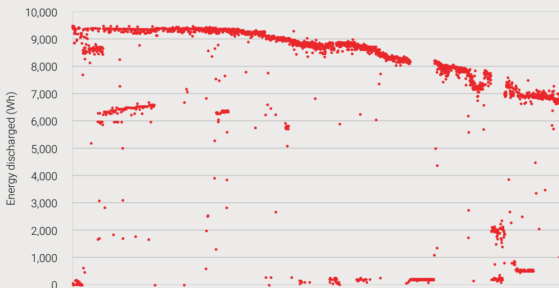
Figure 2: Energy discharged per cycle by the Samsung battery pack
