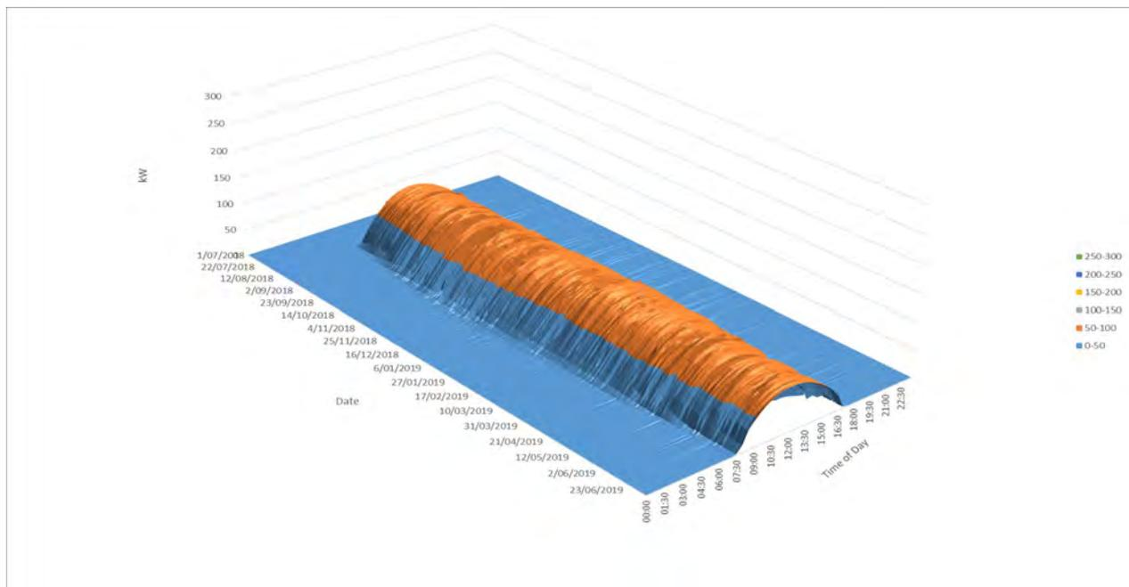
Figure 5: Half-hour averaged solar power (kW) available from Finke solar array over 12 months
