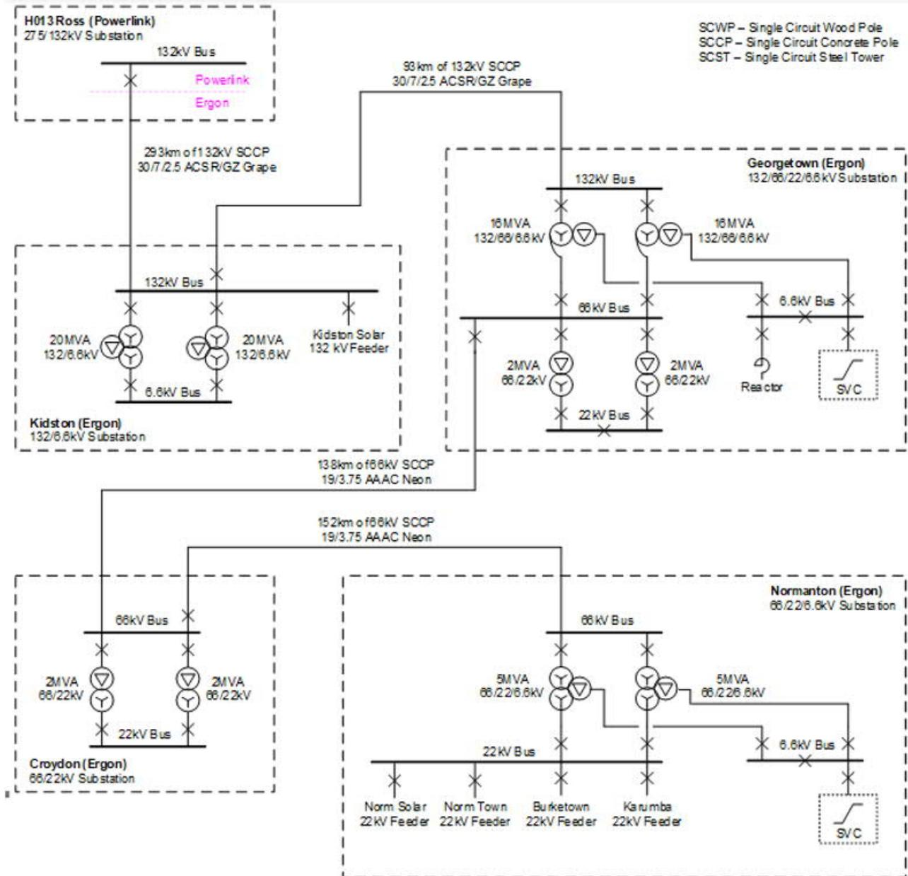
Figure 3-1: Distribution Network Single Line Diagram
