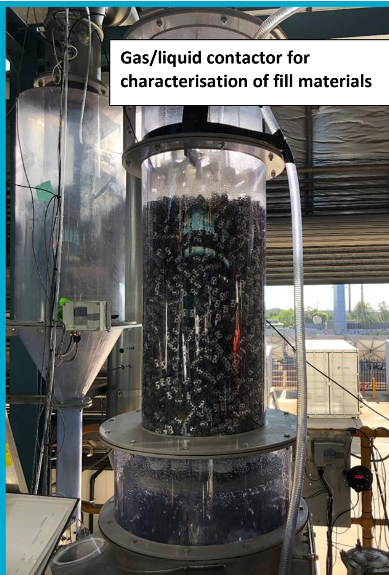
Cooling tower for absorption of CO 2 from the air
