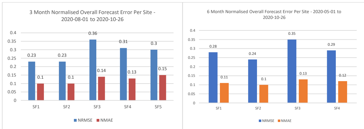
Figure 4 Normalised overall forecast error per site over the last three months (left) and six months (right) for the best model at each site
