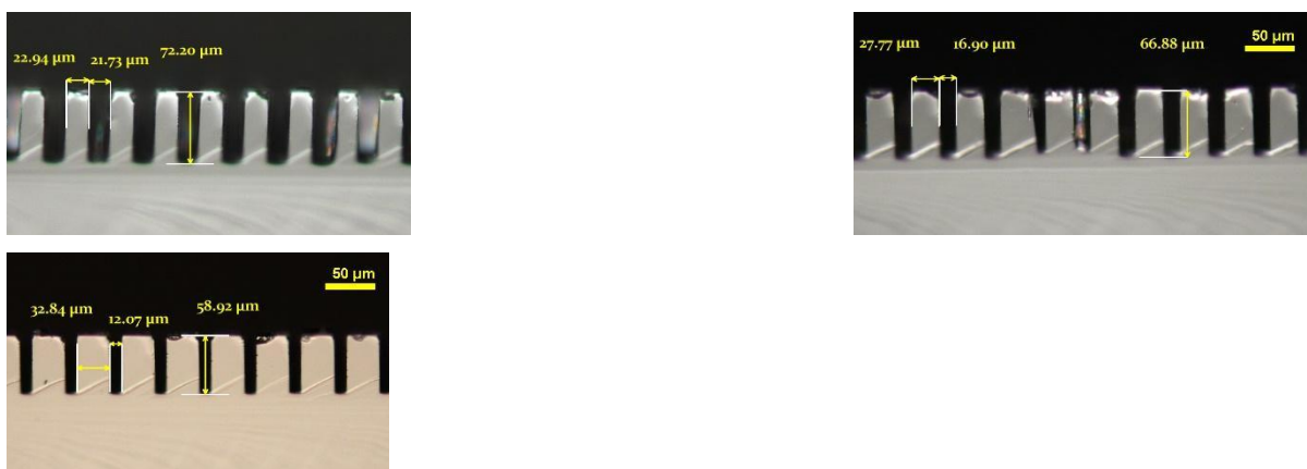
Figure 2: Grooves in GaAs after 30 minutes of ICP/RIE method for groove widths of about 20 (left), 15 (centre) and 10 \mu\text{m} (right).
