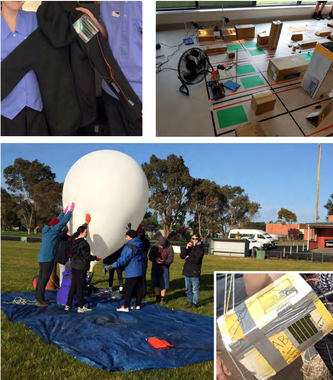
Figure 6.35.7: Images of some of the experimentations conducted by students. (a) OPV modules sewed onto a jacket at Kingston State College, QLD. (b) OPV modules incorporated into an urban design at Casey Tech School, VIC. (c) OPV modules adhered to the payload of a high-altitude balloon at Mount Lilydale Mercy College, VIC.
