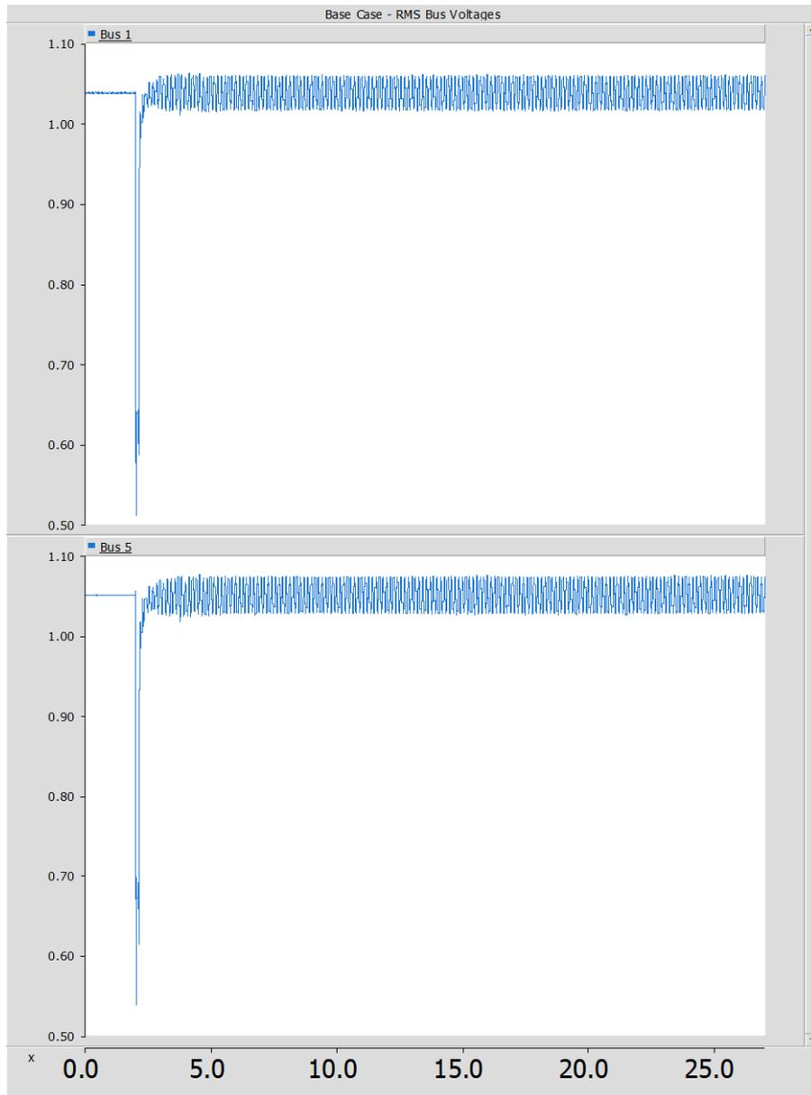
Figure 3 - Un-damped voltage oscillations with inadequate system strength
