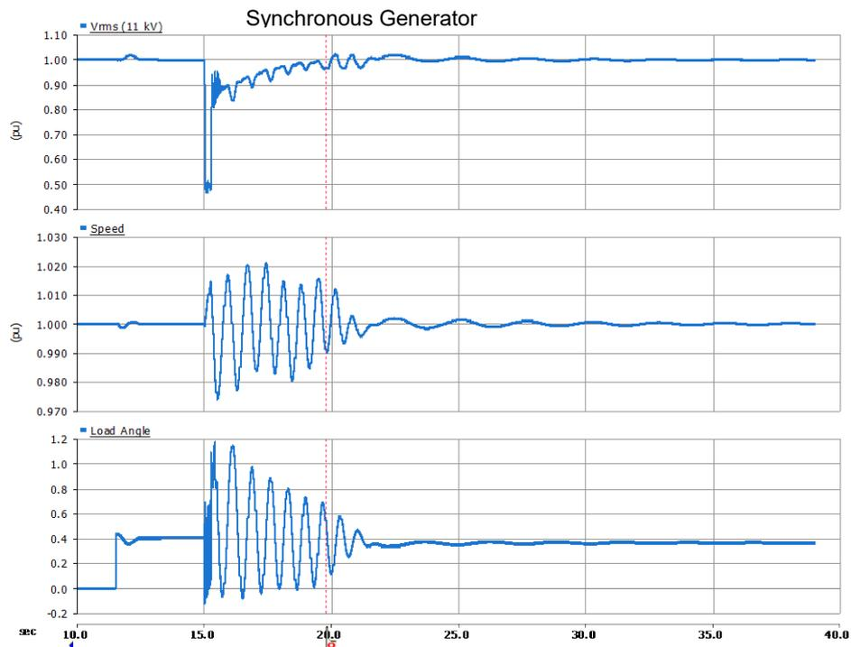
Figure 9 - Nearby synchronous generator remains stable only if both renewable plants reduced to 80% (pre-contingent) and tripped after the fault
