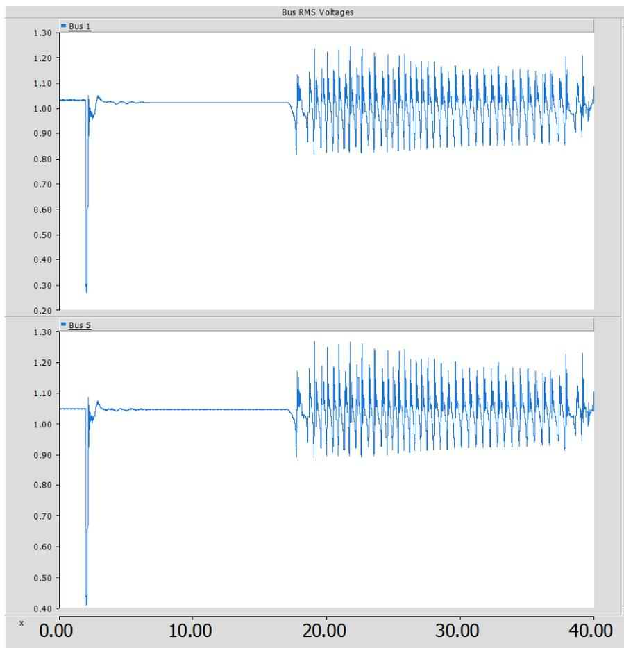
Figure 14 - Grid Bus Voltages, without coordination between the grid forming battery and renewable plants
