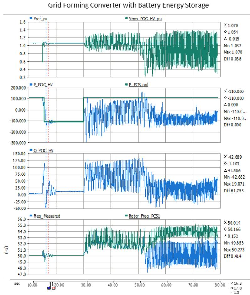
Figure 15 - Grid forming battery's voltage, active and reactive power without coordination with the renewable plants
