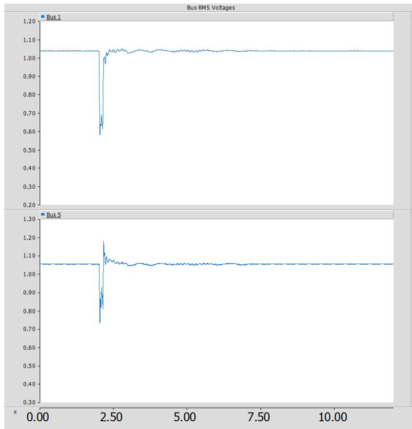
Figure 4 - Grid Bus voltages with a synchronous condenser at Bus 5
