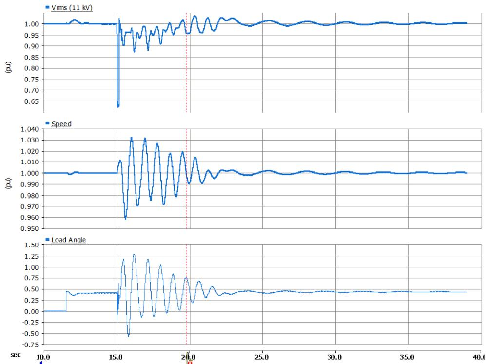
Figure 11 - Nearby Synchronous Generators with proposed synchronous condenser at Bus5 (at least one renewable plant has to be tripped)
