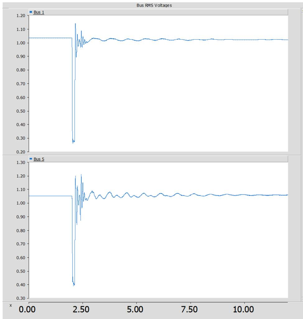
Figure 8 - Grid Bus voltages remain stable only if both renewable plants reduced to 80% (pre-contingent) and tripped fast after the fault
