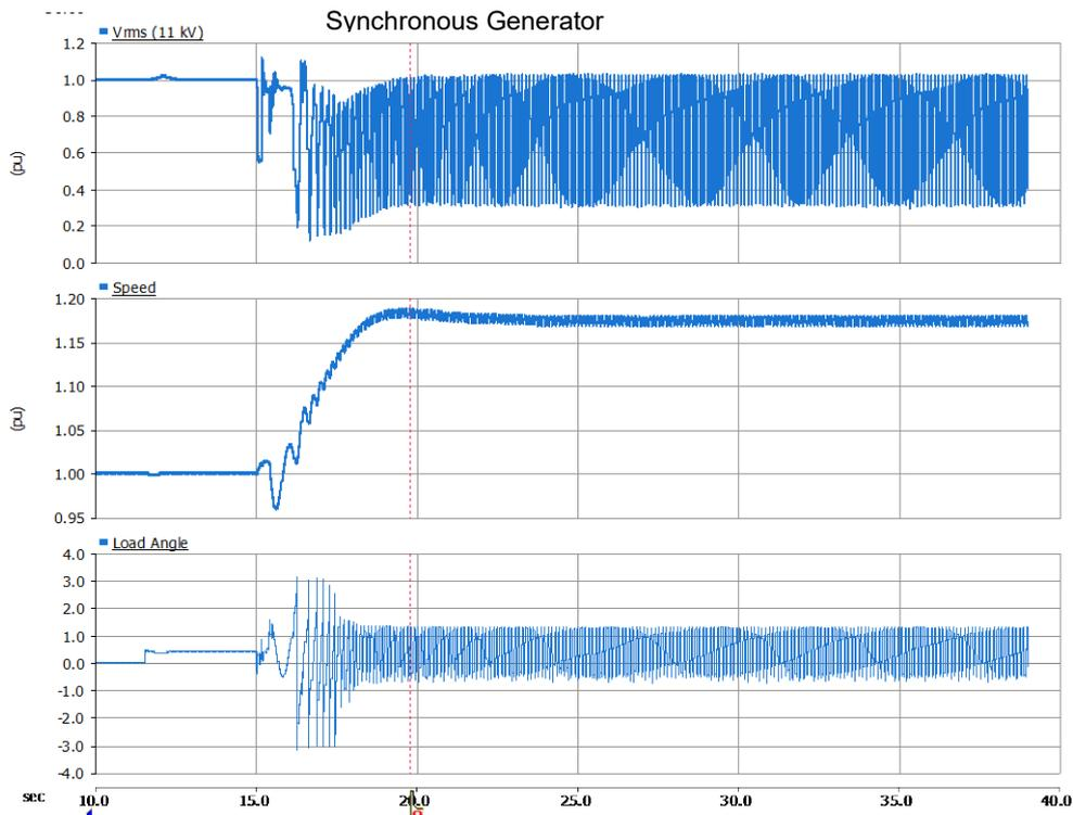
Figure 7 - Nearby Synchronous Generator loses its synchronization
