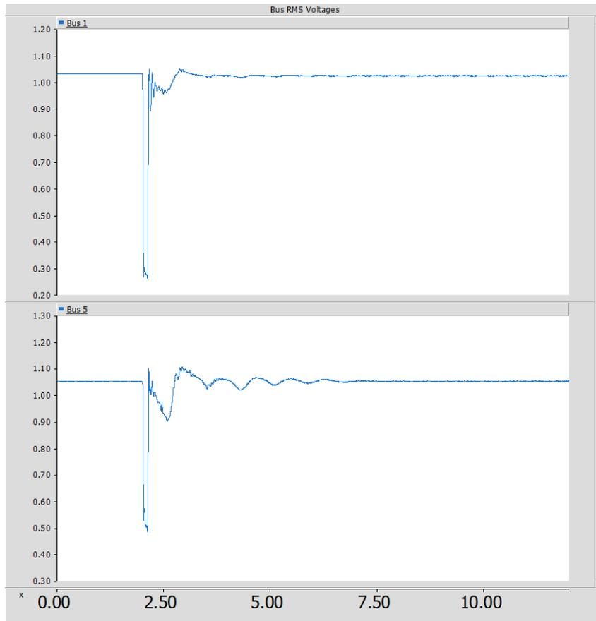
Figure 12 - Grid Bus Voltages with proposed grid forming battery at Bus 5, and with coordinated control between the battery and renewable plants
