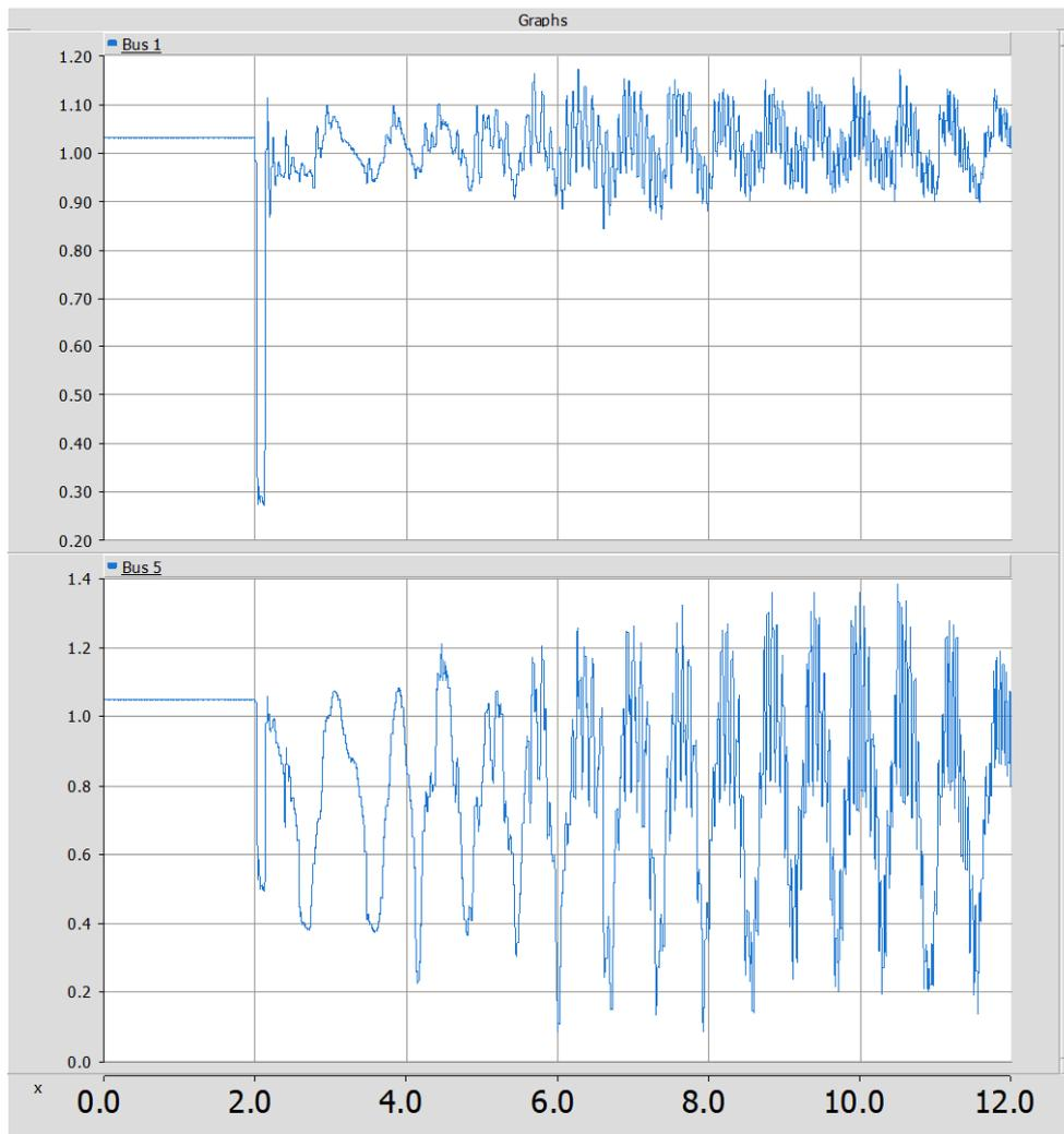
*Figure 6 - Grid Bus voltages collapse after the fault*
