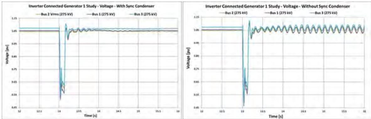
Figure 1 - Example of a stable (left) and unstable (right) response to a disturbance.
