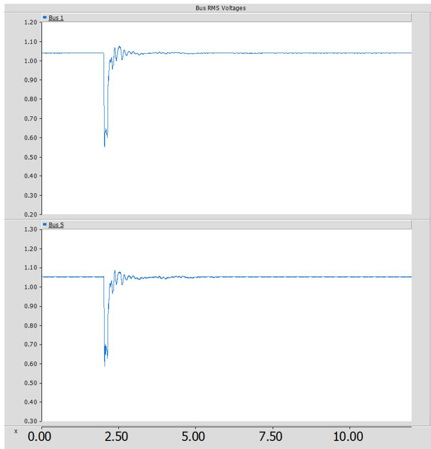
Figure 5 - Grid Bus voltages with a grid forming battery at Bus 5
