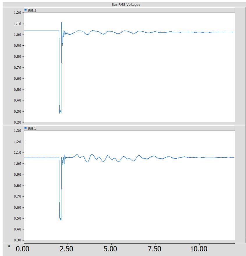
Figure 10 - Grid Bus voltages with proposed synchronous condenser at Bus5 (at least one renewable plant has to be tripped)
