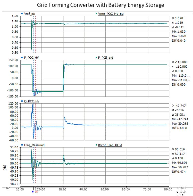
Figure 13 - Grid forming battery's voltage, active and reactive power under coordinated controller with renewable plants
