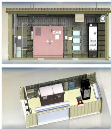
**Figure 4:** (a) basic configuration and operational parameters of equipment for the H2Xport pilot plant. (b) vendor rendering of container housing a NEL electrolyser and Powercell fuel cell.
