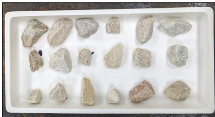
Figure 1- Quartzite Samples Prior to Thermal Cycling
