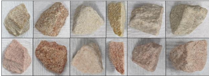
Figure 3- Uncycled (Top) and 50 Cycled (Bottom) Samples
