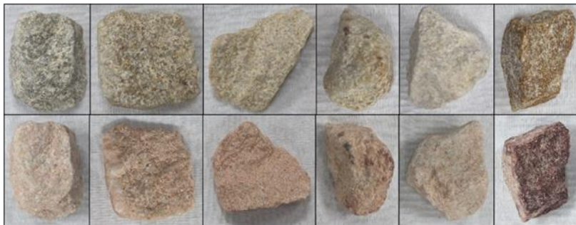
Figure 4- Uncycled (Top) and 100 Cycled (Bottom) Samples
