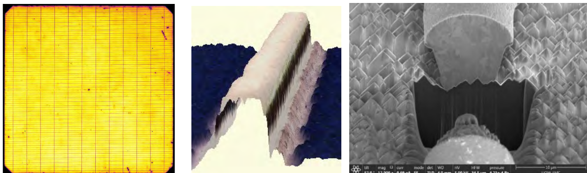
Figure 6: (left) Photoluminescence image of a 25.33% efficient copper-plated solar cell and corresponding surface profile of a copper finger (middle) and SEM image (right) of a selected finger located on the cell.
