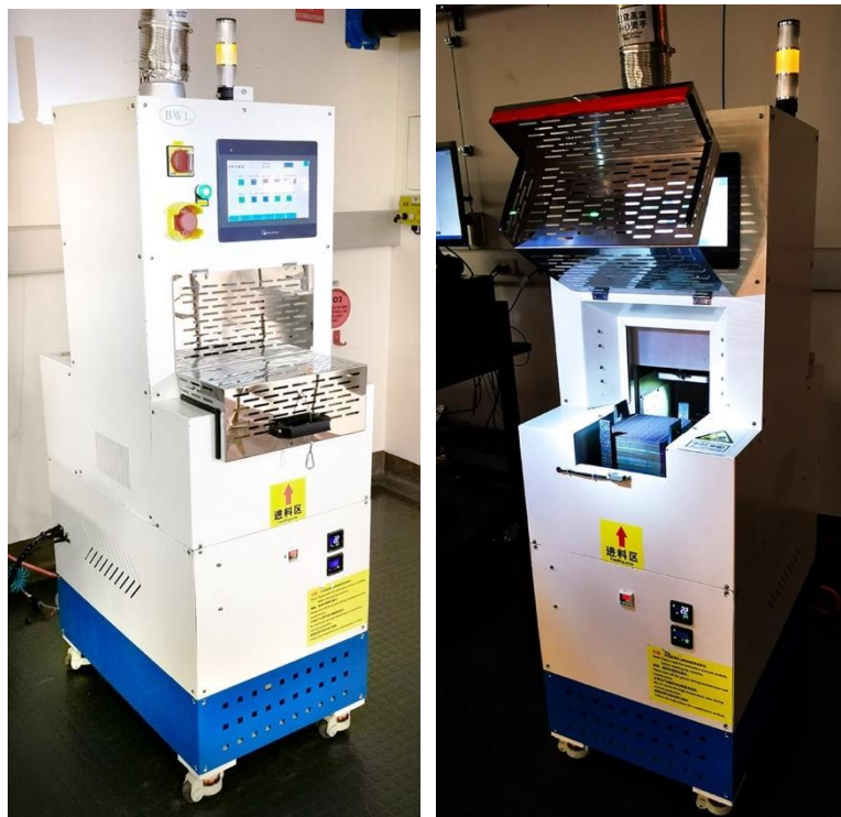
Figure 1: Hydrogen trapping and stability treatment coin-stack prototype tool (a) in operation showing the user interface; (b) showing a stack of 400 cells loaded ready for processing
