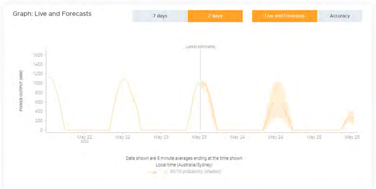
Figure 2-3 A selected excerpt from the Rooftop Solar PV page in the Solcast API Web Toolkit. Data displayed is BtM PV power data, including 48 hours of estimated actuals and 48 hours of forecasts. The P90/P10 ensemble data is shown in the shaded area
