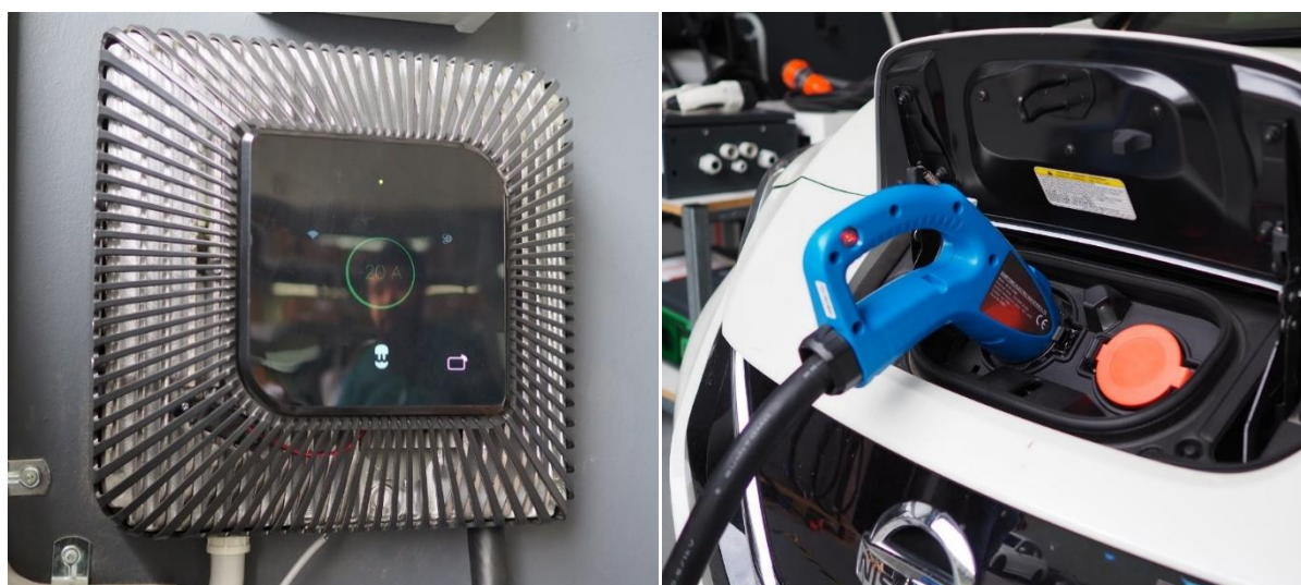
Figure 5: Wallbox Quasar in green 'ready' mode; Charging plug showing red active charging light on the handle.
