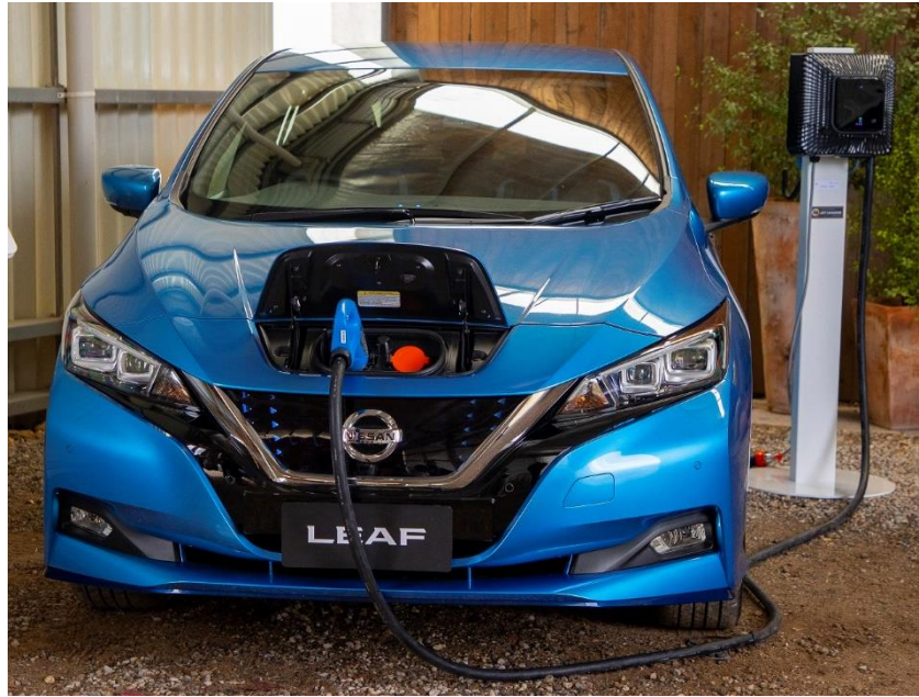
Figure 4: Nissan LEAF charging from a Wallbox Quasar at the CHAdeMO (left) port. The Type 2 (right) port is visible by its orange cap. See also Figure 5 for a close-up view. Source: author.
