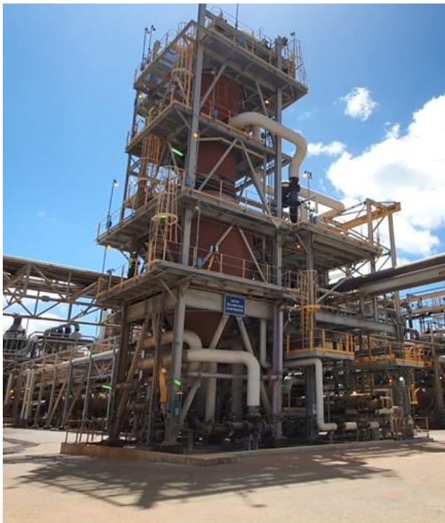
Figure 12 (L) The existing FFE at Wagerup (R) MVR added to the existing FFE
