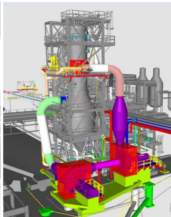
Figure 12 (L) The existing FFE at Wagerup (R) MVR added to the existing FFE
