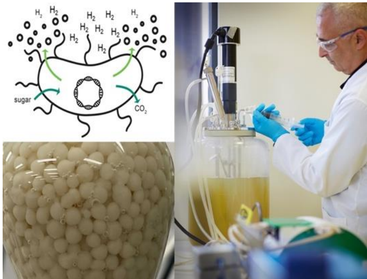
Figure 1: Sugar to hydrogen biocatalyst. A bacterial strain is engineered for hydrogen production and grown to scale using conventional fermentation methods. The bacterial strain is encapsulated and used as a biocatalyst to transform sugar to hydrogen.
