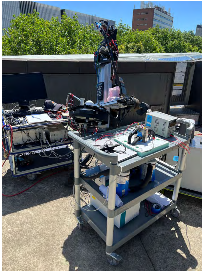
Figure 2b. Photo of the 20 W PVE system for producing green hydrogen with STH efficiencies up to 30%.
