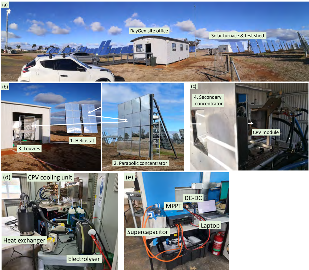
Figure 10. Testing the thermally integrated 1 kW PVE system at RayGen's solar furnace testbed (July 2022): (a) Solar furnace test shed situated at RayGen's Newbridge solar farm; (b) & (c) optics to concentrate sunlight onto the CPV module; (d) thermal integration of PVE via heat exchanger; (e) operator room with DC-DC components and measurement/control computer. When illuminated, the CPV module provides both electricity and heat to the electrolyser.
