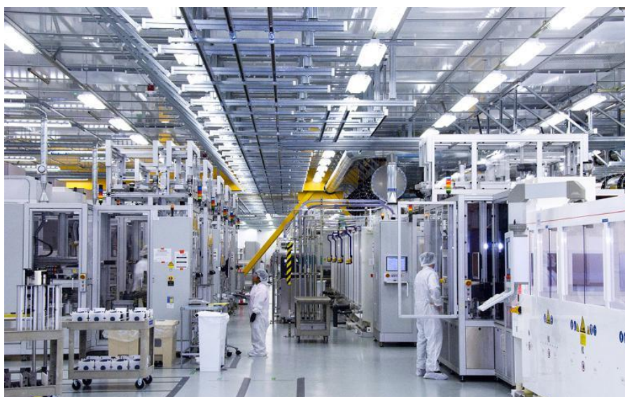
Figure 10: Highly automated solar cell manufacturing line in a clean room facility
