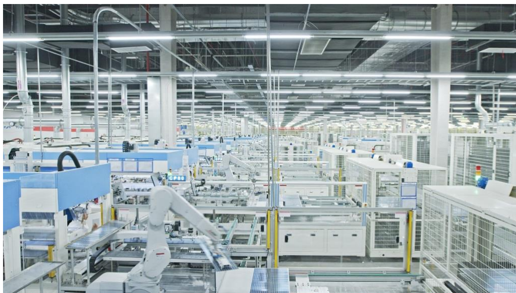
Figure 14: Highly automated solar module assembly facility
