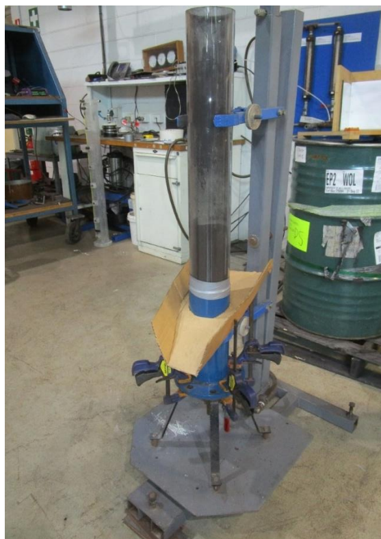
Figure 21: Setup of fluidisation test rig to examine segregation
