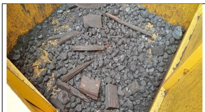
Figure 46– Oversize material bin – 21/3/23
