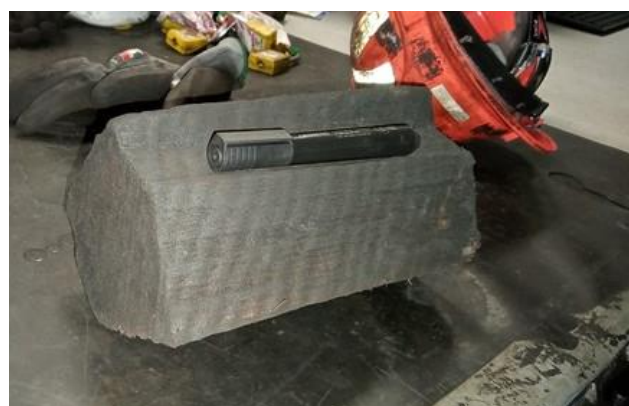
Figure 45 - Timber found blocking biochar flow in Bin 3 – 21/3/23
