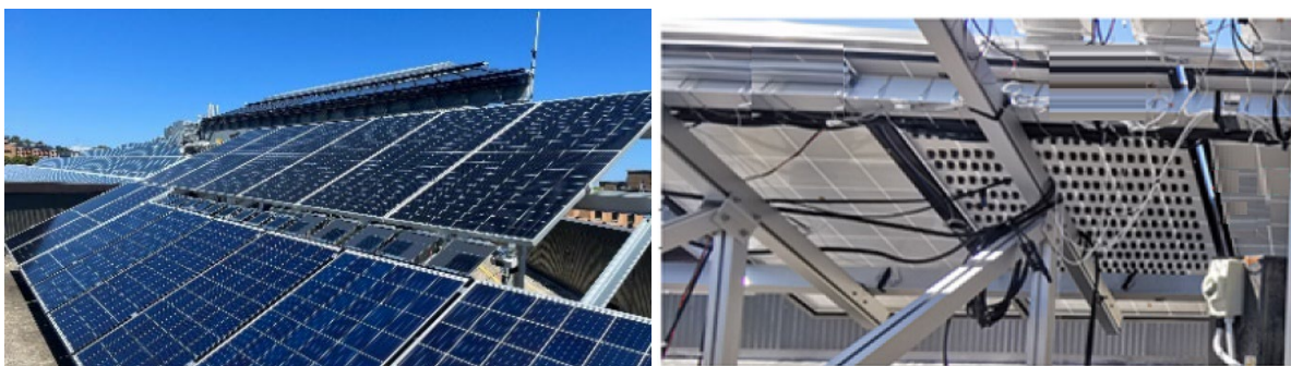
Figure 5: Outdoor test arrays at UNSW from a) the front and b) the rear, with one full sized panel covered in vortex generators.
