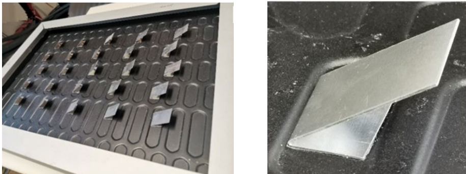
Figure 4. 6-cell test module with both convection cooling using PCI plate and additional VG array to maximise cooling, achieving 4.7°C cooling in field tests.
