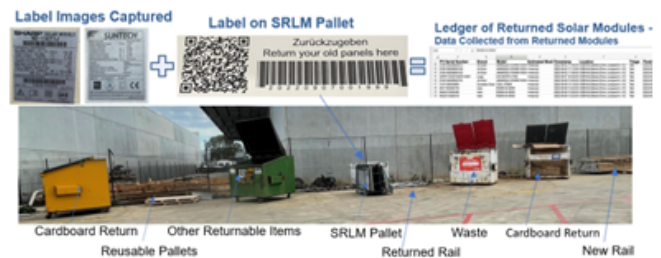
Figure PP4.2.2: Solar Reverse Logistics Model in action at a PV module wholesaler site (the SRLM pallet).
