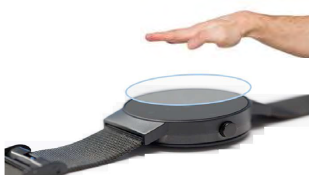
Figure PP2.1.28: Illustration of a transparent solar powered smartwatch with solar-based gesture recognition.
